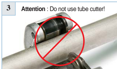
3 Attention : Do not use tube cutter! a) tube cut with tube cutter : heavy burr / bevel cut
