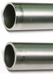
3 Attention : Do not use tube cutter! a) tube cut with tube cutter : heavy burr / bevel cut
