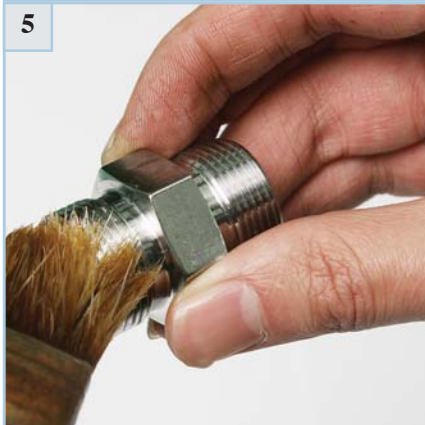
Lubricate thread and cone of fitting body, also cutting ring and thread of nut.
