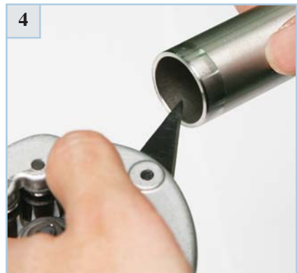
4 Lightly de - burr inside and outside edge. Bevel up to 0.3mm x 45° (0.012" x 45°) permissible.
