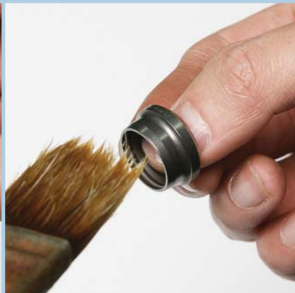
Lubricate thread and cone of fitting body, also cutting ring and thread of nut.
